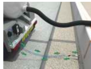
Continuous Ground Loop Monitoring check
